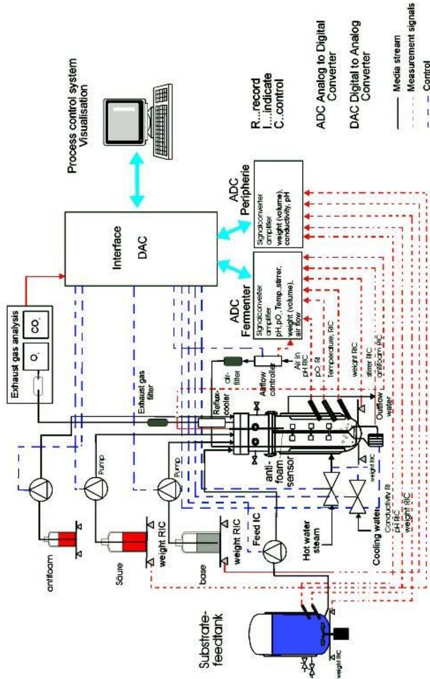
Figure 1. Fermentation processes monitoring and control
